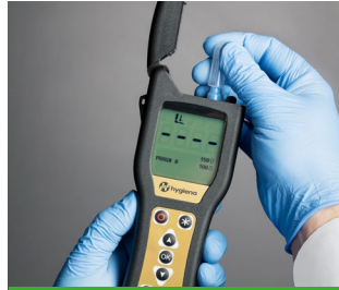
2. Snap Swab & Insert into ATP Meter
